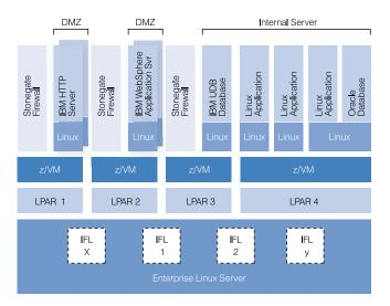
If your security department insists on having separate external firewalls, this can be accomplished very simply by connecting to the ELS using standard NIC adapters as shown in the diagram below.
