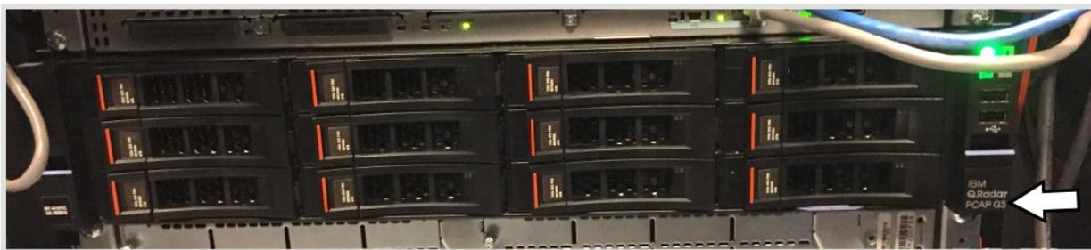
*Figure 1: Front panel of the QRadar Network Packet Capture appliance*
