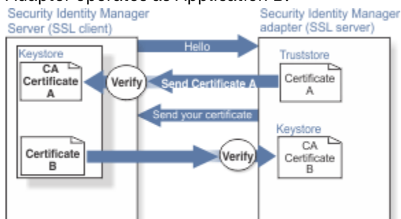
Figure 3. Two-way SSL authentication (client authentication)
