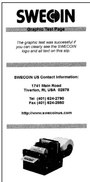
**Figure 6: Diagnostics Test Print Sample**
