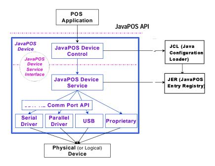
Note: Comm Port API refers to the Java Communications Port API (COM/API) or optionally some other Java communications API that supports hardware device connectivity.
