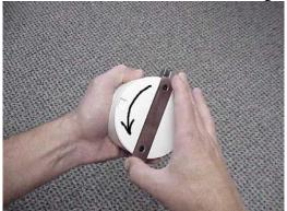
3. Install the batteries. Three 1.5 volt "C" size alkaline batteries are needed for each beacon. The battery orientations are marked inside the beacon.
