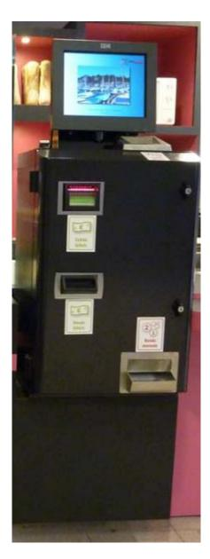
The payment terminal is a device that enables transactions started on a self-service checkout to be completed when the customer wants to pay in cash.
