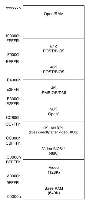
\*Default configuration. If USB legacy support is enabled from system setup, 16K of upper memory is used for the USB stack located from DC000h to DFFFFh. \*\*Video BIOS size may vary depending on various factors. It is currently 48K, and is guaranteed to not exceed 62K in size.
