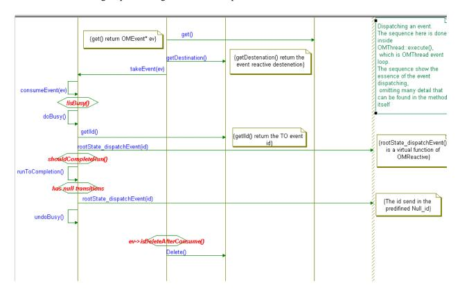
The method OMThread::execute is responsible for the event loop. This sequence diagram shows the main sequence of events that are done inside this method.
