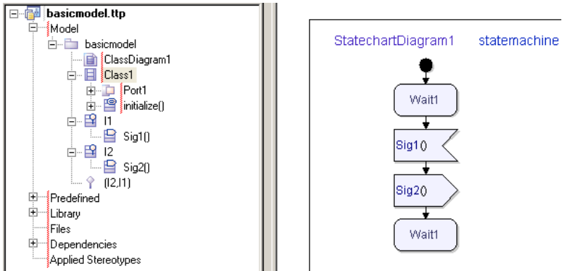
Figure 45: State machine with signal
