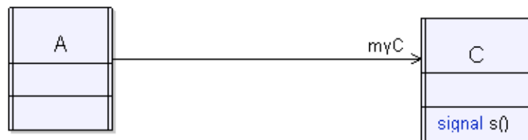
Figure 216: Static structure with explicit addressing.
