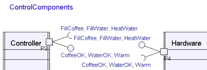
Figure 18: The component diagram with ports and interfaces
