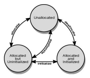
Initially all memory is unallocated. Any reads or writes to unallocated memory will cause Rational Purify to generate a diagnostic message. Once memory is allocated, using malloc/new for instance, it is not yet initialized. Any reads from this memory will generate a Rational Purify diagnostic message. Writing uninitialized memory causes the memory's state to become initialized and it can then be read as well. Calling free/delete causes the affected memory to enter the unallocated state again.
