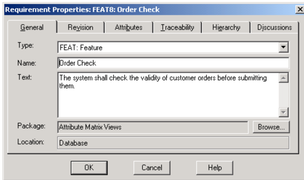
Figure 12: Requirement Text, Attributes, Traceability and Parent-Child settings dialog box
