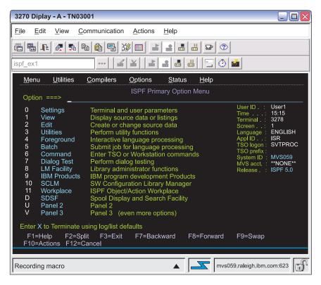
Figure 13. A sample application screen, the ISPF Primary Option Menu
