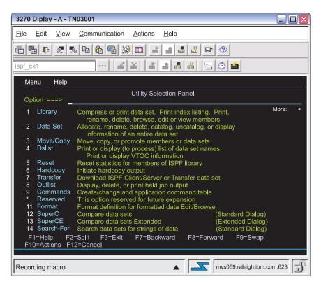
Figure 6. The Utility Selection Panel application screen
