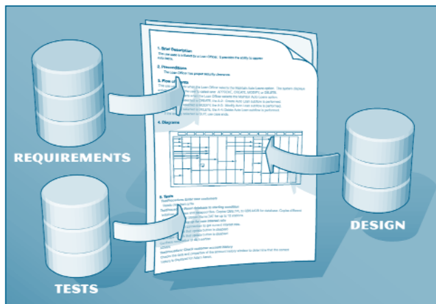
Rational SoDA generates documents by extracting data from your project tool databases.
