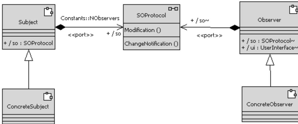
The following diagram shows the structure diagram for ObserverPattern, the top capsule in the system. There is one subject, with some variable number of observers.
