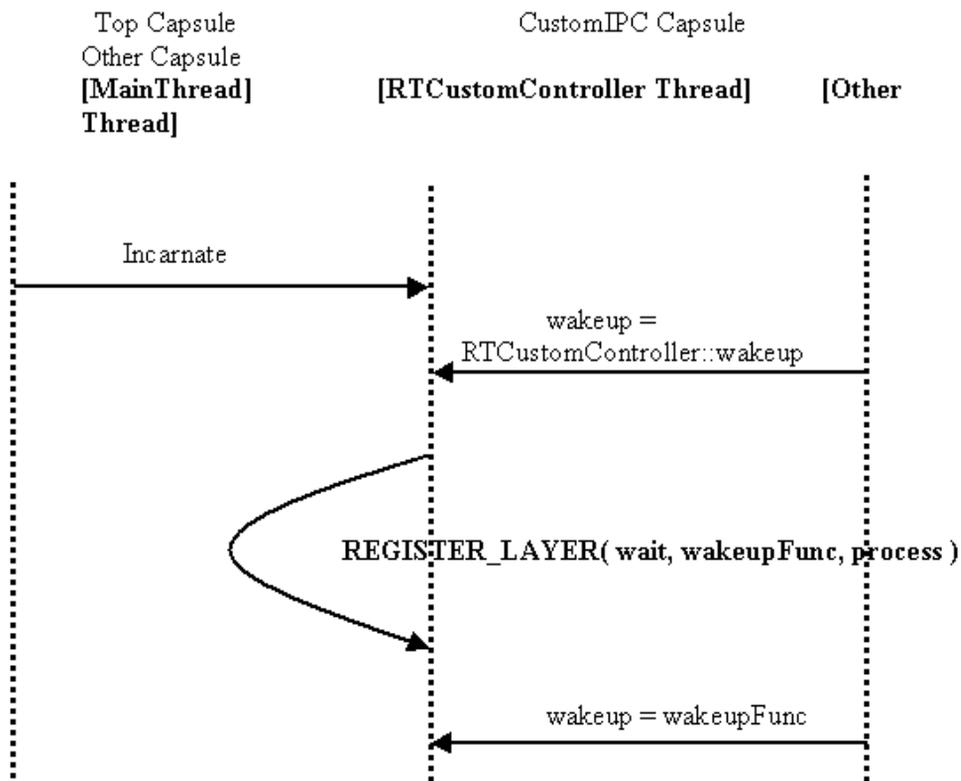
Figure 6: Wakeup control flow of interthread message send involving RTCustomController.
