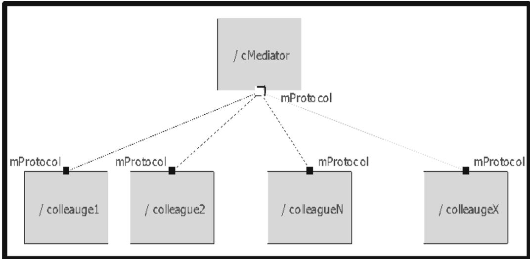
See the MarkI\_Container or MarkII\_Container capsules in the CoffeeMachine\_MoneyBox example model. The MarkI\_Brewer and MarkII\_Brewer capsules function as concrete mediators, while CUSprayer, CUFrontPanel, CUWarmer and CUCashBox function as concrete colleagues.
