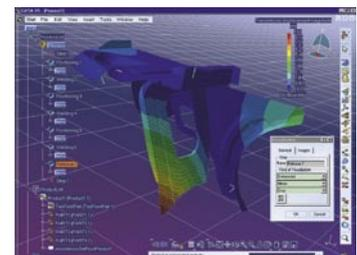
*CATIA – Tolerance Analysis of Deformable Assembly 3 (TAA)*
