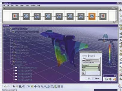
CATIA – Tolerance Analysis of Deformable Assembly 3 (TA3)
