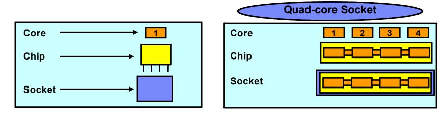
Each chip is plugged into a socket receptacle on the server
