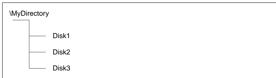
Figure 8. The directory structure for automatic installation from a server. The name MyDirectory is an example only; you must use all the other names.
