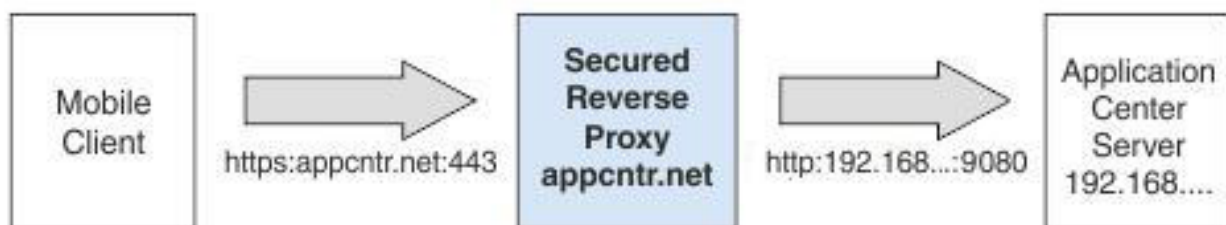
Figure 10. Configuration with secured reverse proxy
