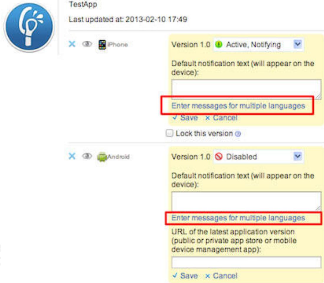
Figure 53. Defining the status of application rules in the IBM Worklight Console
