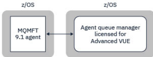
Figure 44. MFT 9.1 agents on z/OS can connect to a queue manager using the CLIENT transport, assuming the queue manager is licensed for Advanced VUE.
