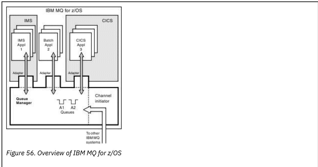
Figure 56. Overview of IBM MQ for z/OS
