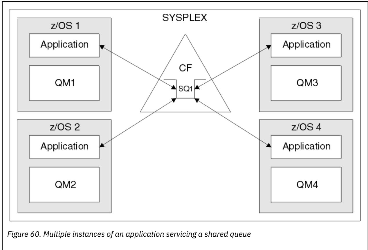
Figure 60. Multiple instances of an application servicing a shared queue
