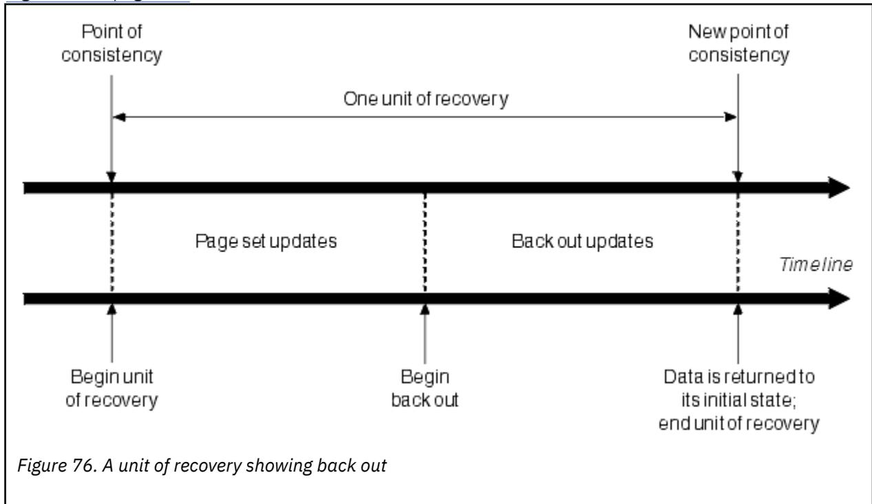
Figure 76. A unit of recovery showing back out
