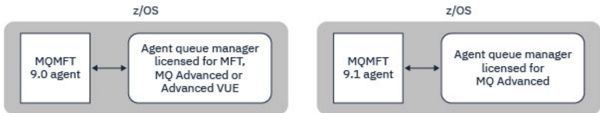
Figure 45. MFT 9.0 agents on z/OS and 9.1 agents that have an agent queue manager licensed for either MFT or IBM MQ Advanced, must connect using the BINDINGS transport.
