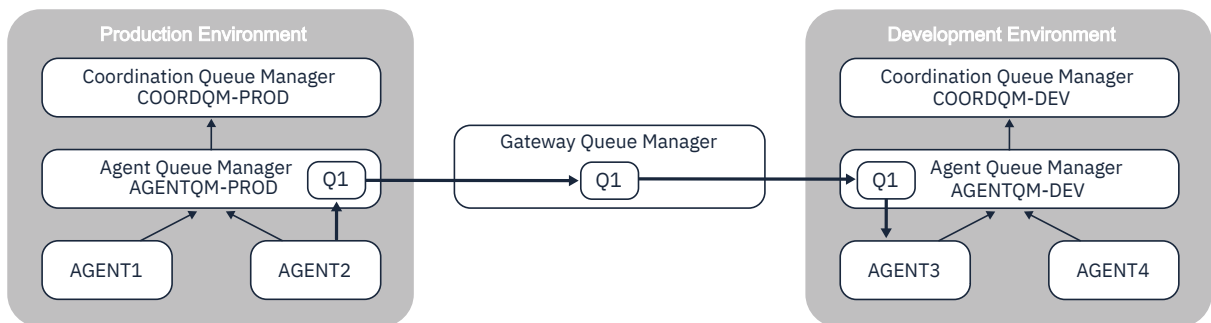
Figure 8. Here, AGENT2 is connected to its agent queue manager AGENTQM-PROD and performs a file-to-message transfer to write a message to a queue called Q1. Q1 is a remote queue, and so the message gets routed via the Gateway Queue Manager and sender/receiver channels to the local queue Q1 on the queue manager AGENTQM-DEV. AGENT3 then performs a message-to-file transfer to get the message and bring it into the Development Environment topology.
