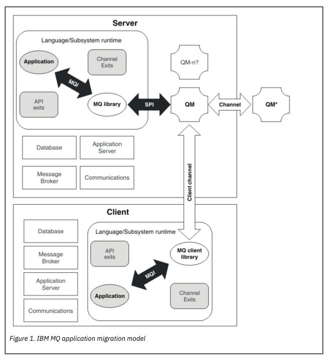
This diagram shows two runtime operating system environments, each of which contains a number of software components, such as databases, application servers, and the language or subsystem run time environment. One environment is called Server, and contains an IBM MQ server and server application. The other environment is called Client, and contains an IBM MQ MQI client application.
