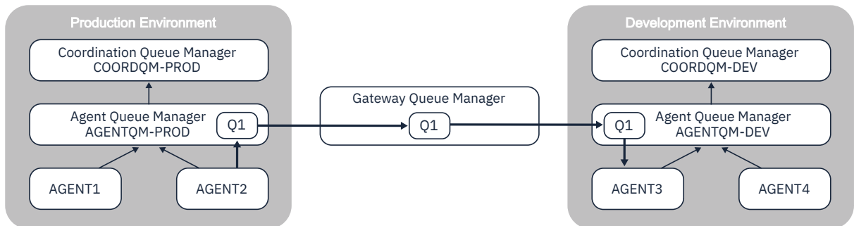
Figure 8. Here, AGENT2 is connected to its agent queue manager AGENTQM-PROD and performs a file-to-message transfer to write a message to a queue called Q1. Q1 is a remote queue, and so the message gets routed via the Gateway Queue Manager and sender/receiver channels to the local queue Q1 on the queue manager AGENTQM-DEV. AGENT3 then performs a message-to-file transfer to get the message and bring it into the Development Environment topology.
