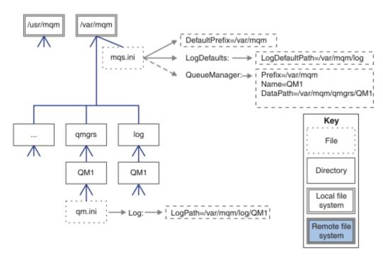
Figure 35. Example default IBM MQ directory structure for AIX and Linux systems
