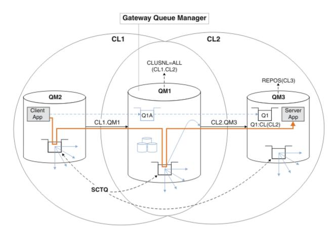
**Note:** The arrows in Figure 12 on page 49 and following figures are of different types. Solid arrows represent message flows. The labels on solid arrows are message channel names. The gray solid arrows are potential message flows from the SYSTEM.CLUSTER.TRANSMIT.QUEUE onto cluster-sender channels. Black dashed lines connect labels to their targets. Gray dashed arrows are references; for example from an MOOPEN call by Client App to the cluster alias queue definition Q1A.
