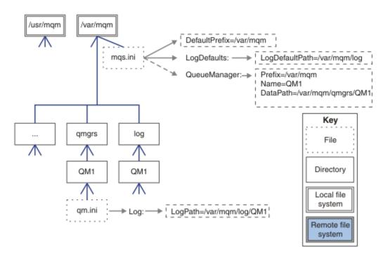
Figure 37. Example default IBM MQ directory structure for AIX and Linux systems
