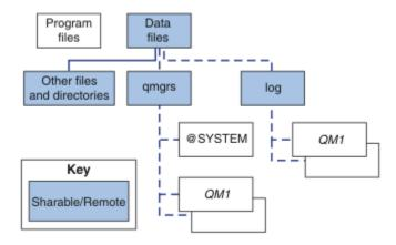
Figure 32. Overall view of IBM MQ directory structure
