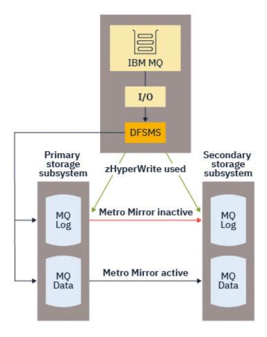
zHyperWrite on IBM MQ, is supported only on the active log data sets.
