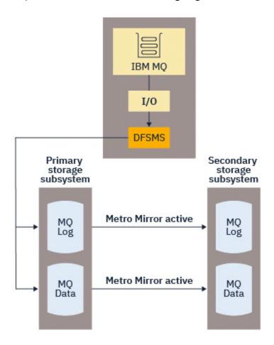
Because both writes to the primary and secondary storage subsystems need to complete before the write returns to IBM MQ, use of Metro Mirror can have a performance impact. You need to balance this performance impact against the availability benefits of using Metro Mirror.
