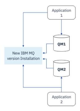
Figure 4. Single\_stage migration: migrated queue managers connected to and applications associated with later version
