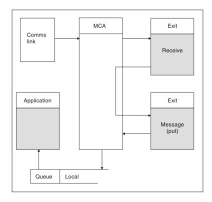
Figure 115. Example of a receive exit at the receiver end of message channel
