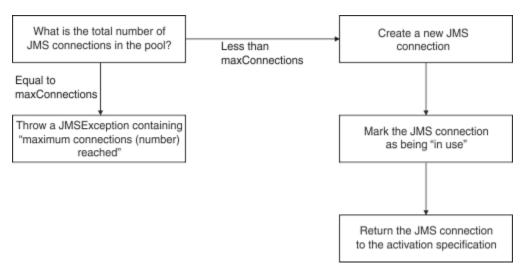
Figure 50. WebSphere Application Server 8.5 - how the connection pool works
