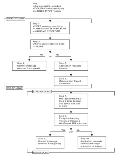
Figure 73. Skipping backout using MQGMO\_MARK\_SKIP\_BACKOUT
