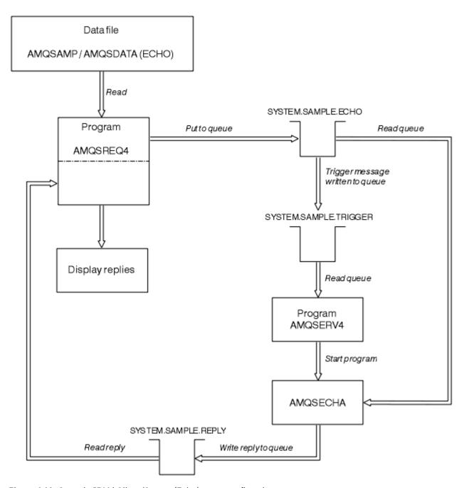
Figure 143. Sample IBM i Client/Server (Echo) program flowchart
