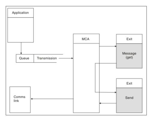
Figure 114. Example of a send exit at the sender end of message channel
