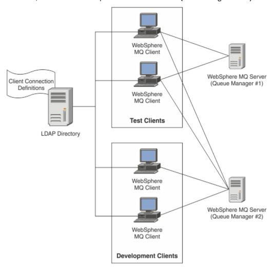
The exit module can look up an LDAP repository, for example, IBM Tivoli Directory Server, to retrieve channel definitions. Using those connection definitions, an IBM MQ client application can establish connection to a queue manager.
