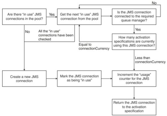
Figure 49. WebSphere Application Server 7.5 and 8.0 - how the connection pool works
