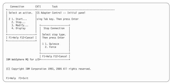
Figure 13. Stopping a connection from the CKQC initial panel
