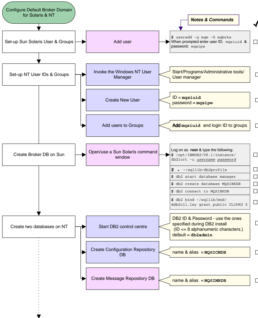
Figure 7. Configuring a simple broker domain
