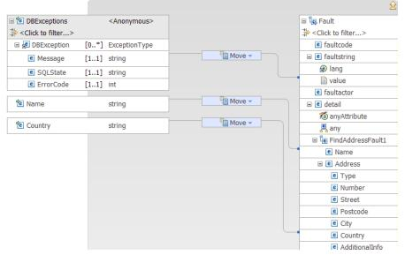
7. Set the cardinality index for the database element **Message** to 1 in the Properties tab of the **Move** transform.
