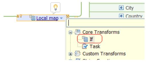
You get an **If** condition with a red exclamation mark connected to two input elements and one output element.
