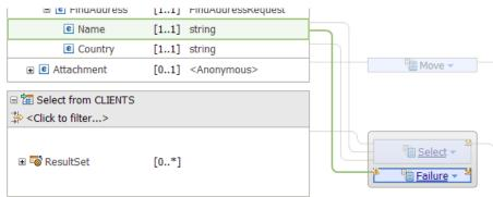
**3**. Connect the message assembly element **Country** to the **Failure** transform. The following figure shows the element **Country** connected to the **Failure** transform:
