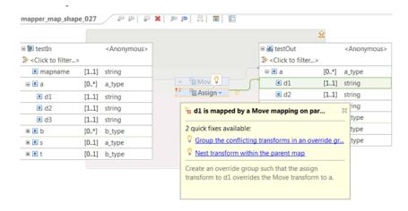
The transforms contained in the overrides group are applied after the parent transform is applied:
