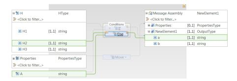
Define a **Move** transform between **H2** and **a**. This operation defines the transformation logic that the **Else** transform performs.
