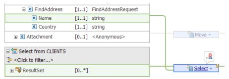
5. Connect the message assembly element **Country** to the **Select** transform. The following figure shows the element **Country** connected to the **Select** transform:
