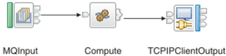
4. On the MQInput node, set the Queue name property (on the **Basic** tab) to TCPIP.TASK16.IN1 .
