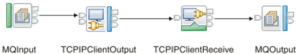
5. On the MQInput node, set the Queue name property (on the **Basic** tab) to TCPIP.TASK19.IN1.
