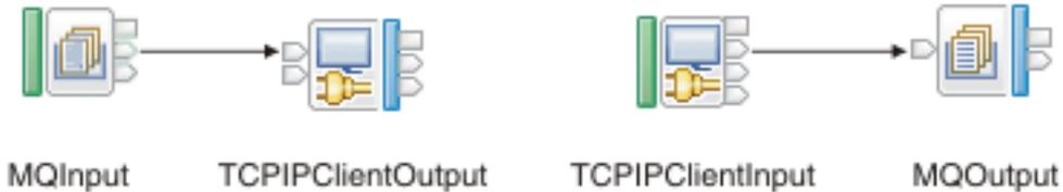
4. On the MQInput node, set the Queue name property (on the **Basic** tab) to TCPIP.TASK7.IN1.
