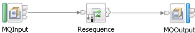
5. On the MQInput node, specify the source of input messages for the node by setting the Queue name property (on the **Basic** tab) to the name of an IBM MQ queue, from which the MQInput node retrieves messages. For example: RESEQ.TASK1.IN1.
