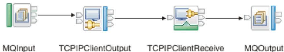
5. On the MQInput node, set the Queue name property (on the **Basic** tab) to TCPIP.TASK6.IN1.
