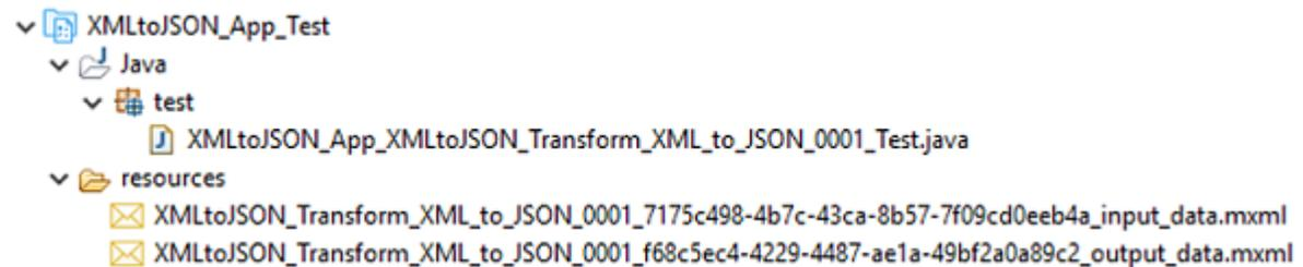
Figure 10. Objects generated by the Create Test Case wizard
