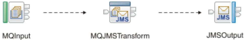
1. An MQInput node receives a message from an IBM MQ queue.
