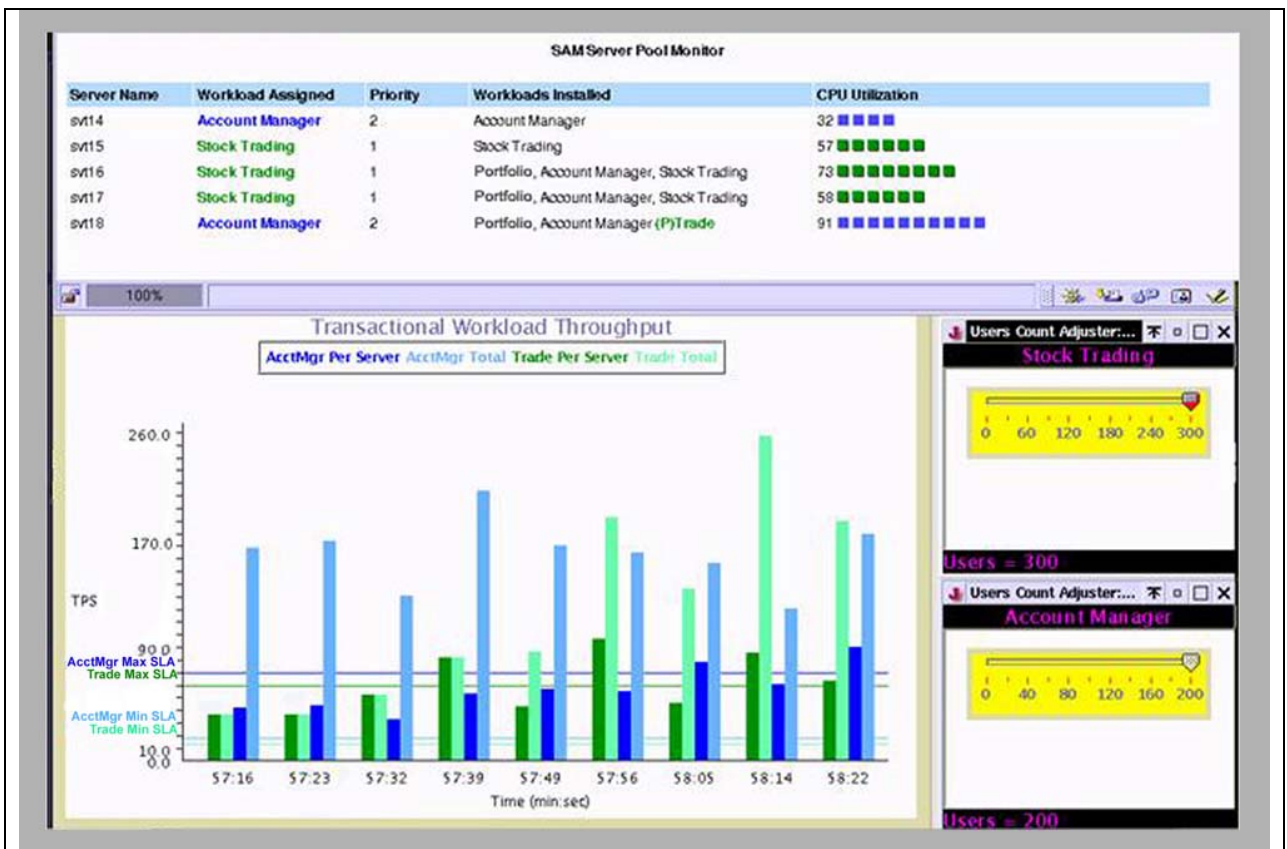
Figure 4. Max SLAs are exceeded; Server Allocation is about to provision an application to Server 18
