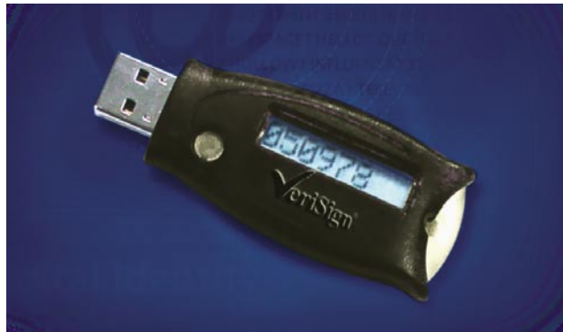
Figure 18. Secure token capable of OTP and PKI authentication.
