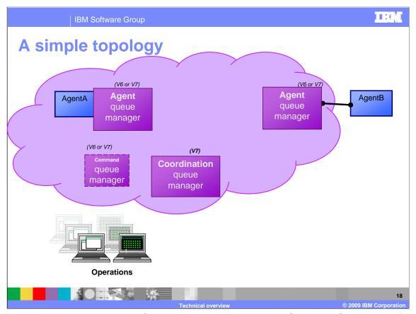
This simple topology shows an MQ network with a simple WebSphere MQ File Transfer Edition configuration. The purple cloud represents the WebSphere MQ network with the purple boxes identifying WebSphere MQ queue managers defined on specific machines within the network.
