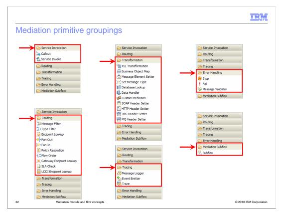
This slide introduces the various mediation primitive groupings. There are various ways that mediation primitives can be organized or classified. In WebSphere Integration Developer, they are categorized into broad groupings based on the primary function of the primitive.
