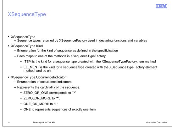
In the XML API, sequence types are represented using XSequenceType objects. XSequenceType objects can represent the same set of sequence types as the SequenceType syntax defined in XPath 2.0. XSequenceType objects are created through the XSequenceTypeFactory interface. XSequenceTypeFactory has several methods for creating XSequenceType instances.
