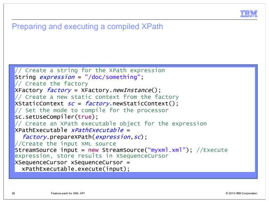
Here is a basic example of preparing and executing a compiled XPath expression. Notice how the XStaticContext interface is used to setUseCompiler to true.
