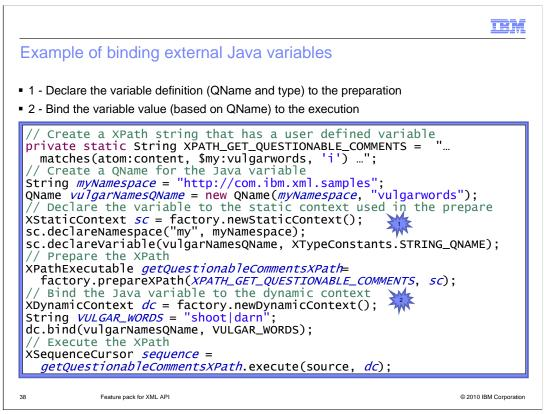
For XSLT and XQuery, variables must be declared in the stylesheet or query itself and thus should not be re-declared in the static context. However, XPath variables need to be declared in the static context. The example here shows the declaration of the variable in the static context and the binding of the variable value in the dynamic context.
