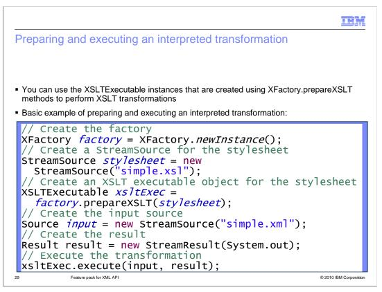
You can use the XSLTExecutable instances that are created using XFactory.prepareXSLT methods to perform XSLT transformations. The example on this page shows a basic example of preparing and executing an interpreted transformation.
