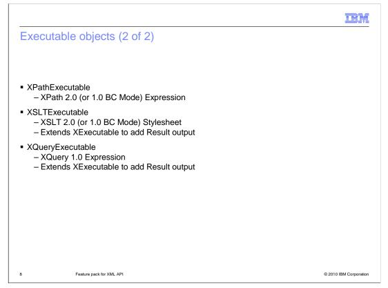
**XPathExecutable** extends <u>XExecutable</u> and represents a prepared XPath expression. All XPathExecutable objects are thread safe. This interface is intentionally empty and you should refer to the XExecutable for available methods.
