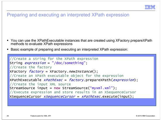
You can use the XPathExecutable instances that are created using XFactory.prepareXPath methods to evaluate XPath expressions. The example here shows a basic example of preparing and executing an interpreted XPath expression. XPath expressions can be passed to the XFactory.prepareXPath method using a JAXP StreamSource object or using a plain Java string object. The resulting XPathExecutable instance is thread safe and can be reused to evaluate an XPath expression on multiple XML input documents.
