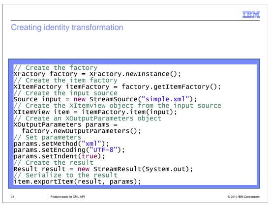
The example on this slide shows how to create an identity transformation. Notice the use of XItemView and the setting of parameters for the output.
