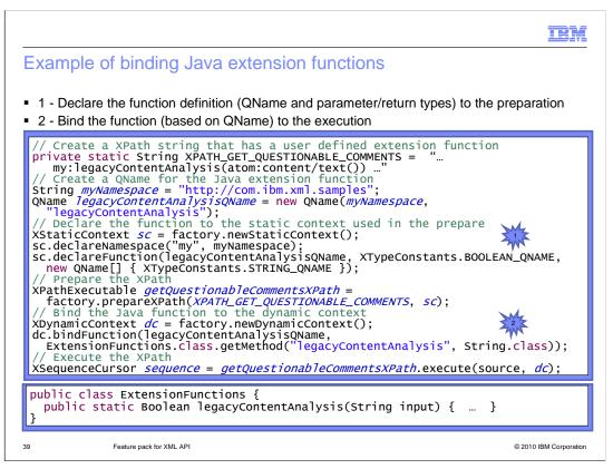
The example here shows how to extend the XML programming model by binding a Java extension function. First you will declare the function definition in the static context, then you will bind the function in the dynamic context.
