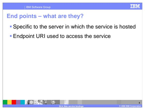
When a service is exposed over the SCA Web service binding, the service endpoint is specific to the server in which the service is hosted. Clients use this endpoint URI to access the service. In some cases, you may want clients to indirectly reference the service by using a proxy server as the service endpoint. For example, a proxy server is required to implement clustered Web service binding endpoints. To enable clients to use a proxied endpoints, there are two ways to do this:
