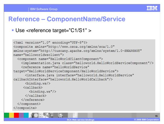
This example shows the use of a reference specifying the target attribute to resolve the service endpoint (Example: <reference
