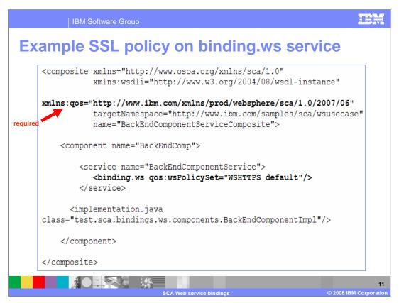
This example shows how SSL policy is applied to **binding.ws** service. Reference side is similar. The key point here is that the **xmlns** for qos: is required.
