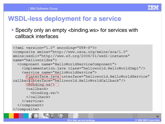
This example is showing how to use WSDL-less deployment **for a Service**. For services with callback interfaces specify only an empty <binding.ws>. This is because The callbackinterface requires its own binding.ws for the callback since a callback is implemented as a bi-directional service. Therefore it has its own service and reference defined in SCDL. Additionally, the callback also must define its interface.
