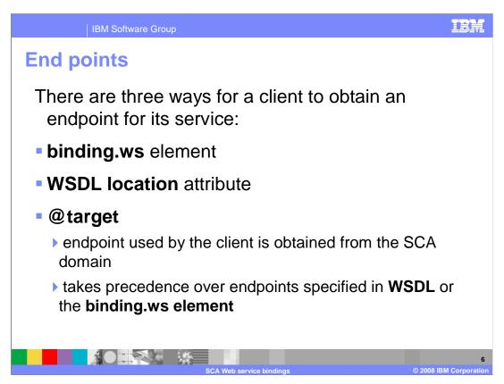
There are three ways for a client to obtain an endpoint for its service: through **binding.ws** element, through WSDL location attribute, and through target annotation. When target annotation (@target) is used, the endpoint used by the client is obtained from the SCA domain. It takes precedence over endpoints specified in WSDL or the binding.ws element. Therefore when using @target annotation you do not need to specify any reference endpoints.
