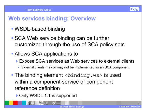
Web services binding is a WSDL-based binding; that means that it either references an existing WSDL binding or allows one to specify enough information to generate one. When an existing WSDL binding is not referenced, WSDL binding can be generated. SCA Web service binding can be further customized through the use of SCA Policy Sets.
