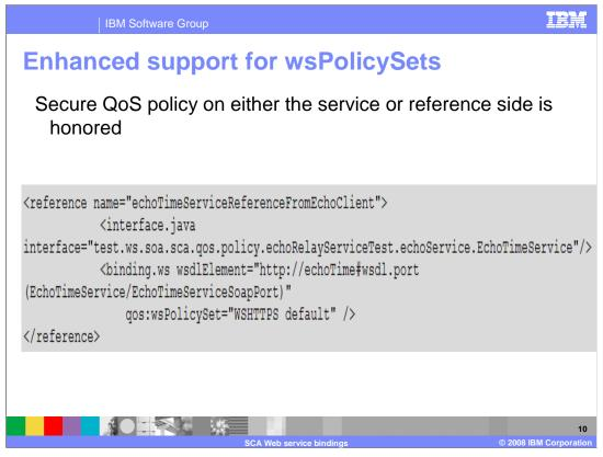
In the past, services exposed to the Web services binding were always available over both secure and non-secure endpoints. Now, if a service is described with a QoS policy that requires SSL, the service will not be available on a non-secure endpoint.
