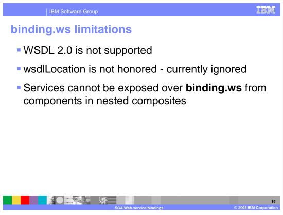
Here are some Web service binding limitations for SCA feature pack; WSDL 2.0 is not supported, which implies wsdl.endpoint is not supported, wsdlLocation is not honored, this is currently ignored and services cannot be exposed over **binding.ws** from components in nested composites.
