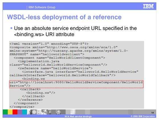
This example is showing how to use WSDL-less deployment for a Reference.
