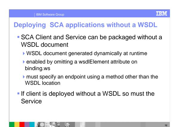
SCA Client and Service can be package without a WSDL document. This is enabled by omitting a wsdlElement attribute on binding.ws and not packing a WSDL document with your contribution. In this scenario, the WSDL document will then be generated dynamically at runtime. Clients must specify an endpoint using a method other than the WSDL location attribute since WSDL does not exist.
