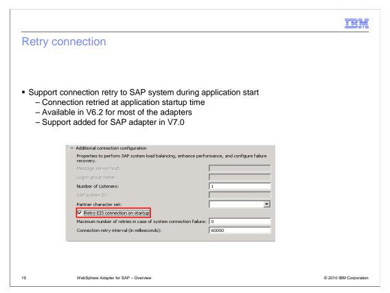
Retry connection is an option that you can enable when configuring the adapter using the external service wizard. When enabled, during application start, the adapter will retry connecting to the SAP system based on the number you configure for maximum number of retried property.
