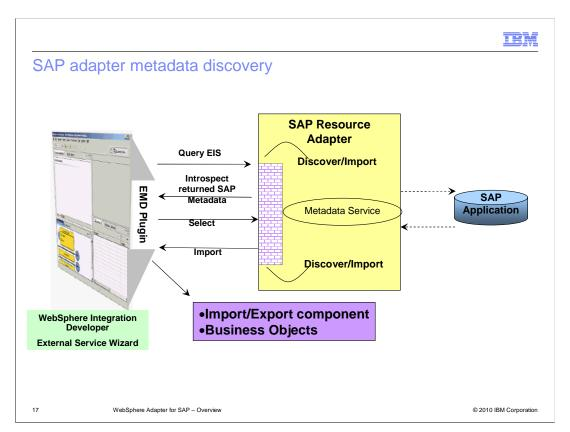
This diagram shows the interaction between the External Service wizard in WebSphere Integration Developer and the Enterprise Metadata Discovery (EMD) support classes within the SAP adapter. It also shows the end to end flow of interaction from the tool to the adapter to the SAP application to create the artifacts for the outbound and inbound requests to and from SAP.
