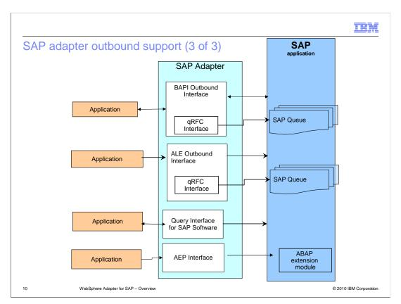
This diagram shows the high level flow and the components in outbound calls. The various interfaces that the adapter supports for outbound are shown in the diagram above. You can use the adapter to make BAPI calls, exchange data using IDocs over ALE interface, interact directly with application tables using query interface for SAP software interface or can call ABAP handlers when using the advanced event processing interface.
