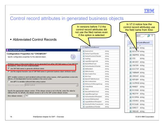
In prior versions selecting the option to "use SAP field names to generate attribute names" for the business objects only resulted in SAP field names being used for the data record and not control record. With V7.0 if you enable this option, both control and data record attributes in the business object will use SAP IDoc field names.
