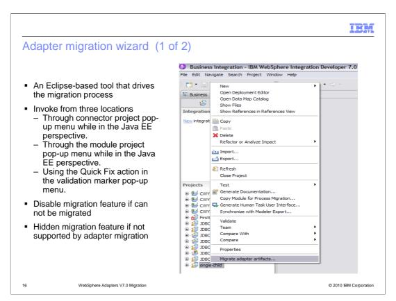
The migration wizard is an Eclipse-based tool that drives the migration process. Its function is driven by the metadata specified at the adapter level and the APIs implemented in the extension plug-in.
