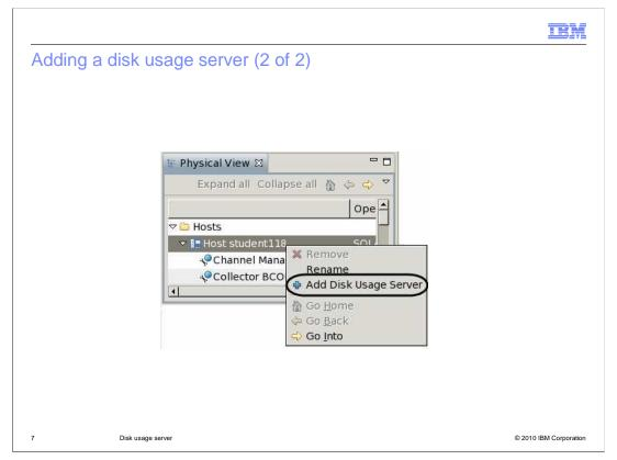
The disk usage server is assigned to a specific host in the Physical view of the Topology editor. You can right-click a specific host name in the Physical view to add the server.
