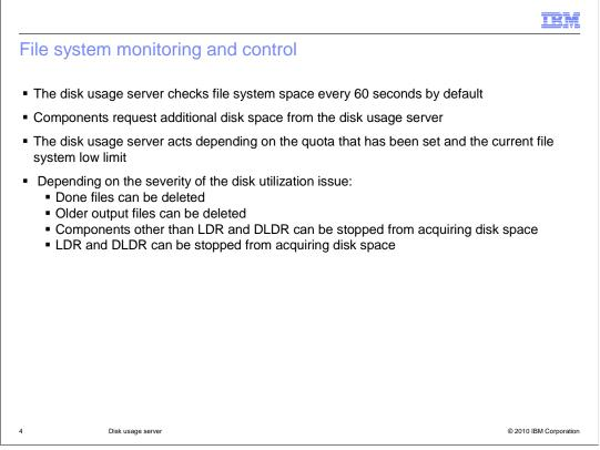
The disk usage server checks file system space every 60 seconds by default. Components request additional disk space from the Disk Usage Sever.
