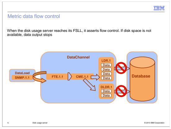
Flow control is asserted when the disk usage server reaches 99% of its quota, or when the file system low limit (FSLL) is met. If not enough space is available to satisfy the quota or FSLL, the disk usage server interrupts operation and stops processing data. Data is never deleted from the **/state** directory to provide disk space.
