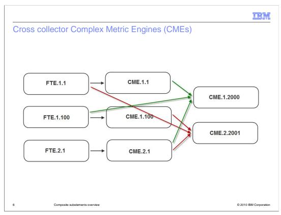
IBM Tivoli Netcool Performance Manager Wireline Component requires a cross collector/channel CME capability. A composite subelement can consist of metric data from many FTEs and CMEs and from many channels. To use CSEs in an installation, at least one cross collector CME must be created.
