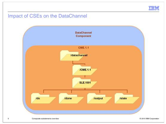
The CME directory path contains a new directory structure between the root directory and the **/do**, **/done**, **/output**, and **/state** directories. The directory structure acquires its name from a concept called Single Label Engine (SLE). There is one SLE directory structure per CME in Tivoli Netcool Performance Manager 1.3 Wireline Component.
