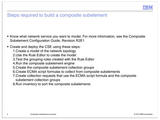
CSE structures are created in Tivoli Netcool Performance Manager Wireline Component using the DataMart Rule Editor. After a structure has been created, Complex Metric Engine (CME) formula files are written in ECMA script language. They are deployed against the composite subelement structure. The formulas that are defined within the file use the composite subelement definitions to navigate the structure and retrieve the appropriate input metrics for their calculations.
