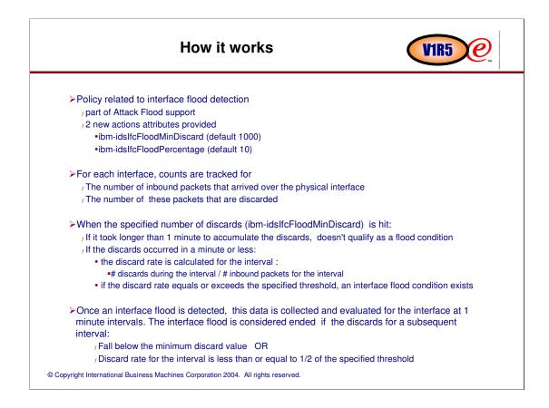
The minimum discard count (ibmidslfcFloodMinDiscard) is the minimum number of discards that must occur in a 1 minute interval before considering a condition an interface flood.
