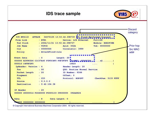
Event data is uses to show the prior hop source ip address, if available. The event data fields is a general usage field that is displayed in hex, EBCDIC and ASCII. The source MAC information is most readable in the EBCDIC format.
