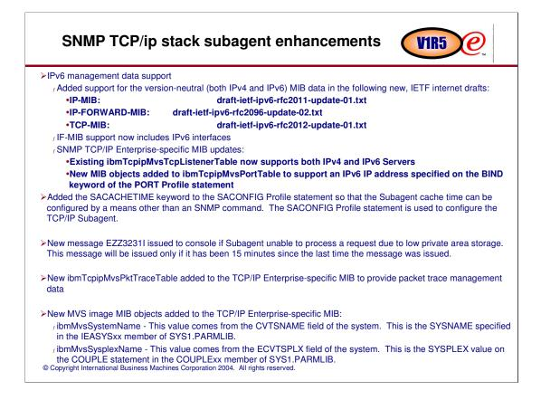
"version-neutral" MIB object definitions are based on SNMP textual conventions defined in the INET-ADDRESS-MIB from RFC 3291 and IETF draft draftietf-ops-rfc3291bis-00.txt.
