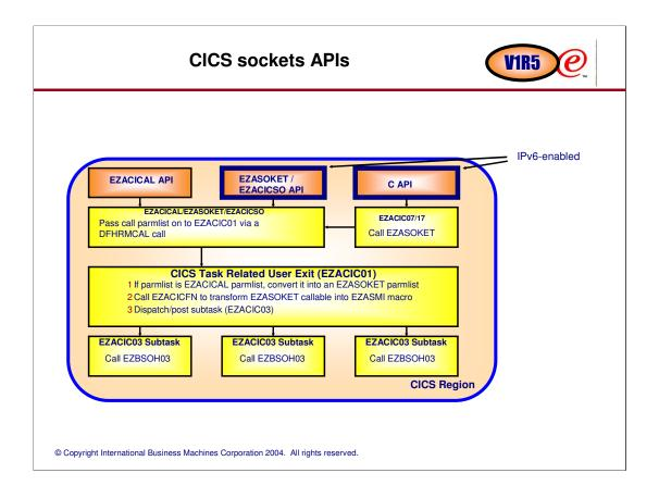
Both CICS C-sockets and Call EZACICAL socket programs are transformed into calls to the sockets extended callable API before the socket calls are passed down to the socket communicating subtasks, making the full CICS socket implementation much more streamlined. The subtasks now only have to do call routing on behalf of the CICS task.
