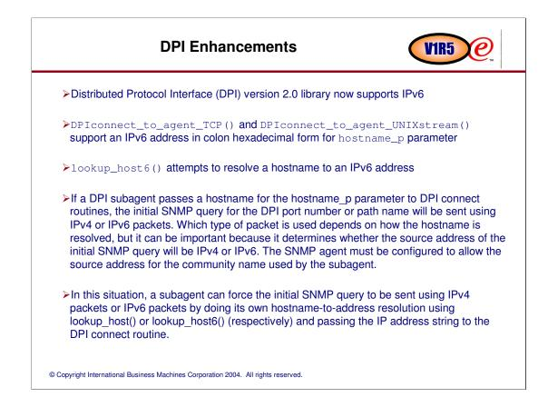
If a DPI subagent passes a hostname for the hostname\_p parameter to DPI connect routines, the initial SNMP query for the DPI port number or path name will be sent using IPv4 or IPv6 packets. Which type of packet is used depends on how the hostname is resolved, but it can be important because it determines whether the source address of the initial SNMP query will be IPv4 or IPv6. The SNMP agent must be configured to allow the source address for the community name used by the subagent.
