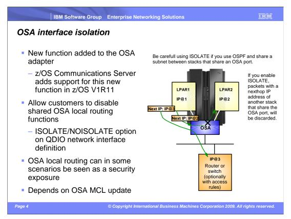
In some environments where strict control over routing between IP nodes must be enforced, the loop-back feature of a shared OSA port can prevent such rules from being enforced. Assume sending an IP packet from LPAR1 to a home IP address of LPAR2 (without VLAN tagging or attached to the same VLAN). In that case OSA will send that packet up to LPAR2 directly without sending it out to the switch. If the switch is there to enforce access rules, that behavior is an issue.
