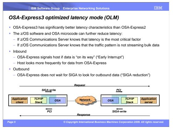
OSA-Express3 and z/OS V1R11 Communications Server are allowing configuration of a new mode of operation for an OSA-Express3 in QDIO mode – optimized latency mode (OLM). When in this mode, several processing improvements are being implemented.
