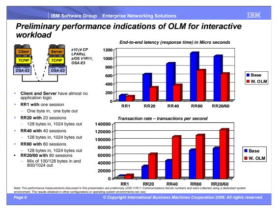
Optimized latency mode is meant for interactive workloads. The maximum number of TCP/IP stacks (LPARs) that can share an OSA adapter operating in OLM mode is limited to four. The general assumption is that customers will use dedicated OSA ports for workloads where they plan to use the OLM capability.
