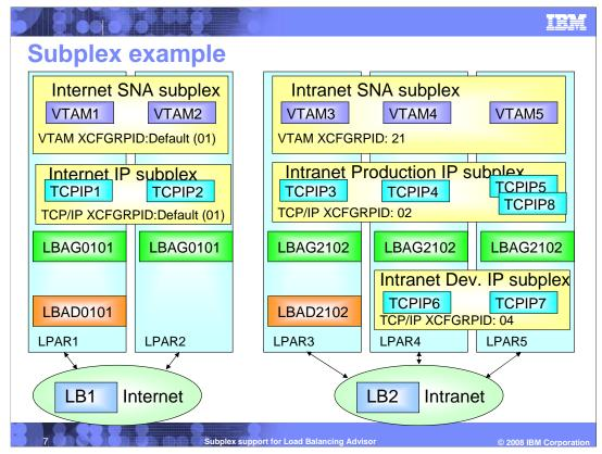
The previous figure is now shown with LBA applications configured to allow external Load Balancers to connect to the Internet IP subplex and the Intranet Production IP subplex.
