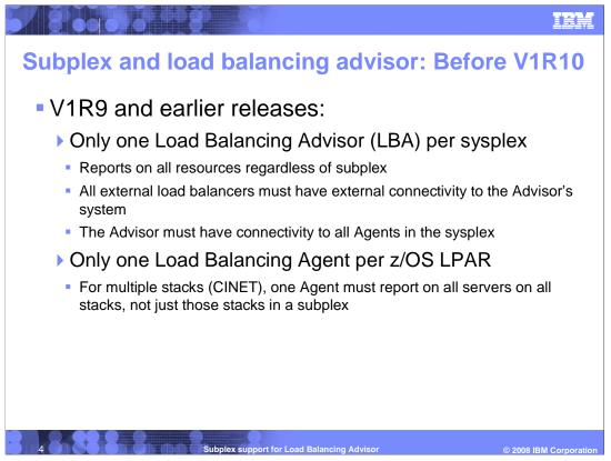
Before z/OS V1R10, the z/OS Load Balancing Advisor and Agent did not formally support the TCP/IP and SNA subplex function that was introduced in z/OS V1R8. While the Load Balancing Advisor and Agents do not explicitly make use of XCF services, they do not fit as neatly into a TCP/IP subplex environment in their pre-V1R10 implementation.
