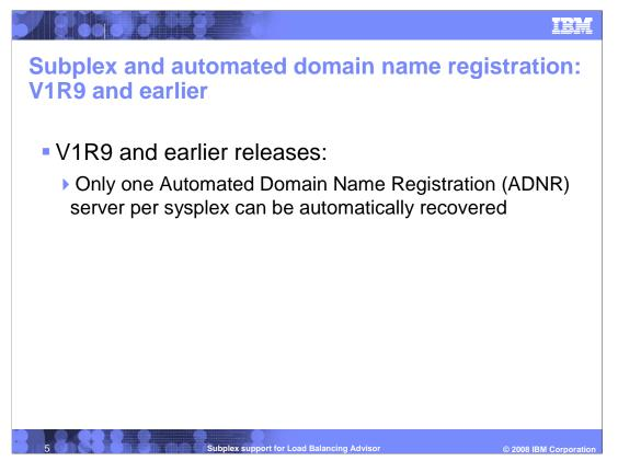
In V1R9, you can start multiple ADNR instances in a sysplex, but only one is recoverable using the automated restart manager (ARM). This inhibits recoverability, particularly in a subplex environment.
