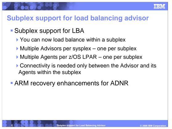
In z/OS V1R10, you can now load balance within a subplex. The Advisor allows multiple instances of itself to be present in the sysplex environment. Each Advisor is configured with the TCP/IP sysplex group name of the subplex that Advisor is handling.
