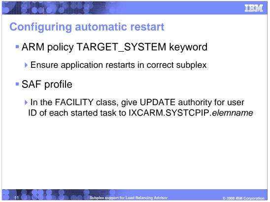
You should define an ARM policy with the TARGET\_SYSTEM keyword to indicate which systems the element can be restarted on in order to ensure that the application is restarted only on a system that is in the same subplex. The Advisor and Agent should be restarted on a system with a VTAM that has been started with the same XCFGRPID (*vv*) and has an available TCP/IP stack with XCFGRPID *tt*.
