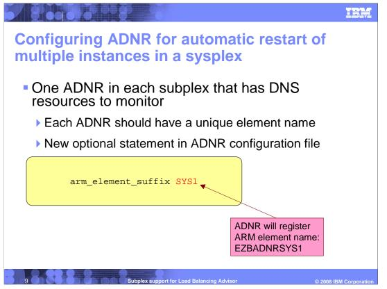
ADNR supports only one connection to an Advisor. If you are using ADNR in a subplexing environment, you will need a separate ADNR instance in each subplex that contains name server resources being monitored by ADNR.
