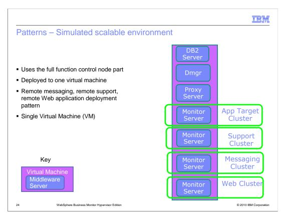
The simulated scalable environment is a pattern that contains the full function control node pattern part. This pattern part includes a DB2 server, a deployment manager, a proxy server, and four WebSphere Business Monitor clusters. There is a cluster defined for the application target, support, messaging and Web applications.
