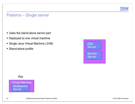
The single server WebSphere Business Monitor pattern is a single virtual machine that is composed of the operating system, a DB2 server, and a WebSphere Business Monitor installed with a single stand-alone server instance defined.
