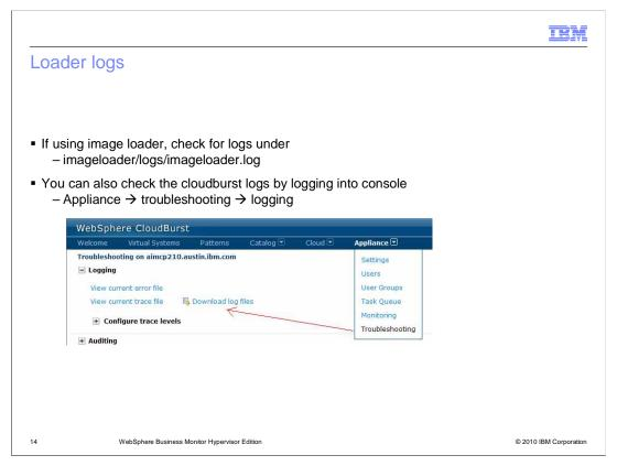
When using the image loader tool to upload the virtual image to the WebSphere CloudBurst catalog, logging information is captured in the imageloader/logs/imageloader.log file at the location where you started the image loader script file.
