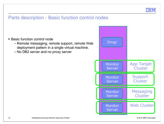
The second of the more complex pattern parts is the basic function control node.
